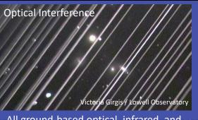
All ground-based optical, infrared, and radio observatories are affected, but NSF's brand new \$400M Vera Rubin Observatory, with its wide field of view, could have streaks in 30% of images (and up to 90% at twilight). The current technical goal of 7th magnitude brightness for satellites is driven by Rubin Observatory science needs.
