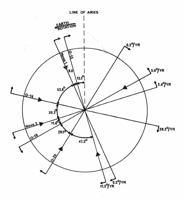
Fig 3. Orbits of the Transit and Nova Satellites on 31 December 1984, Viewed from above the North Pole
