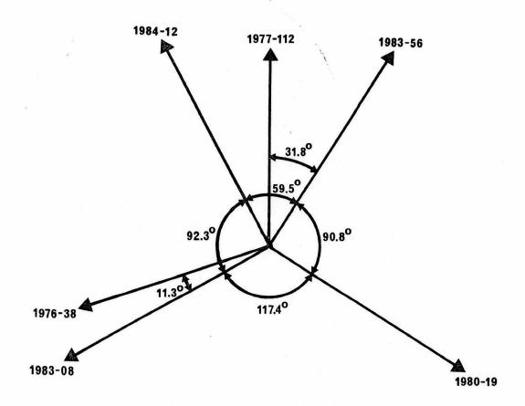
Fig 1. Relative Spacing of the Orbital Planes of the Ocean Surveillance Satellites
