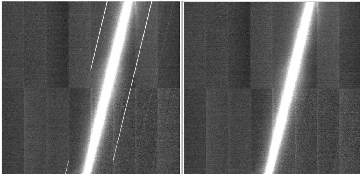
**Figure C.1.** Crosstalk: (*left*) a trail of brightness comparable to that expected from a LEOsat at 550 km generates parallel “ghost” trails due to electronic crosstalk in the sensor and electronics. These crosstalk effects are nonlinear and may be removed in LSSTCAM down to near the background noise level with a pixel processing algorithm, providing the satellite is fainter than about 7th magnitude (*right*).
