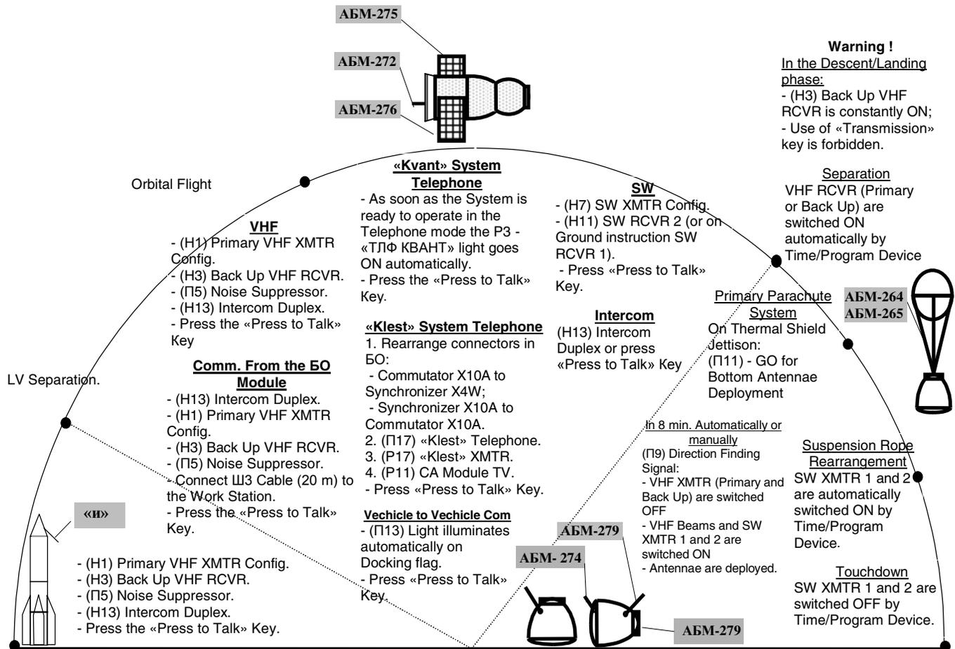
Fig. 3. (Soyuz Spacecraft Flight Phase Communication Arrangement)
