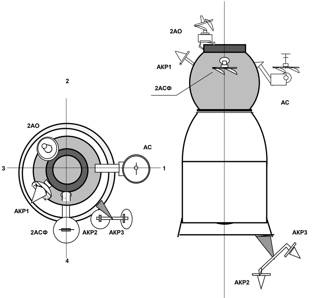
Fig.1. (PTCC System Antennae Layout)
