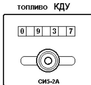
**Fig. 12. Propellant Quantity Meter**
