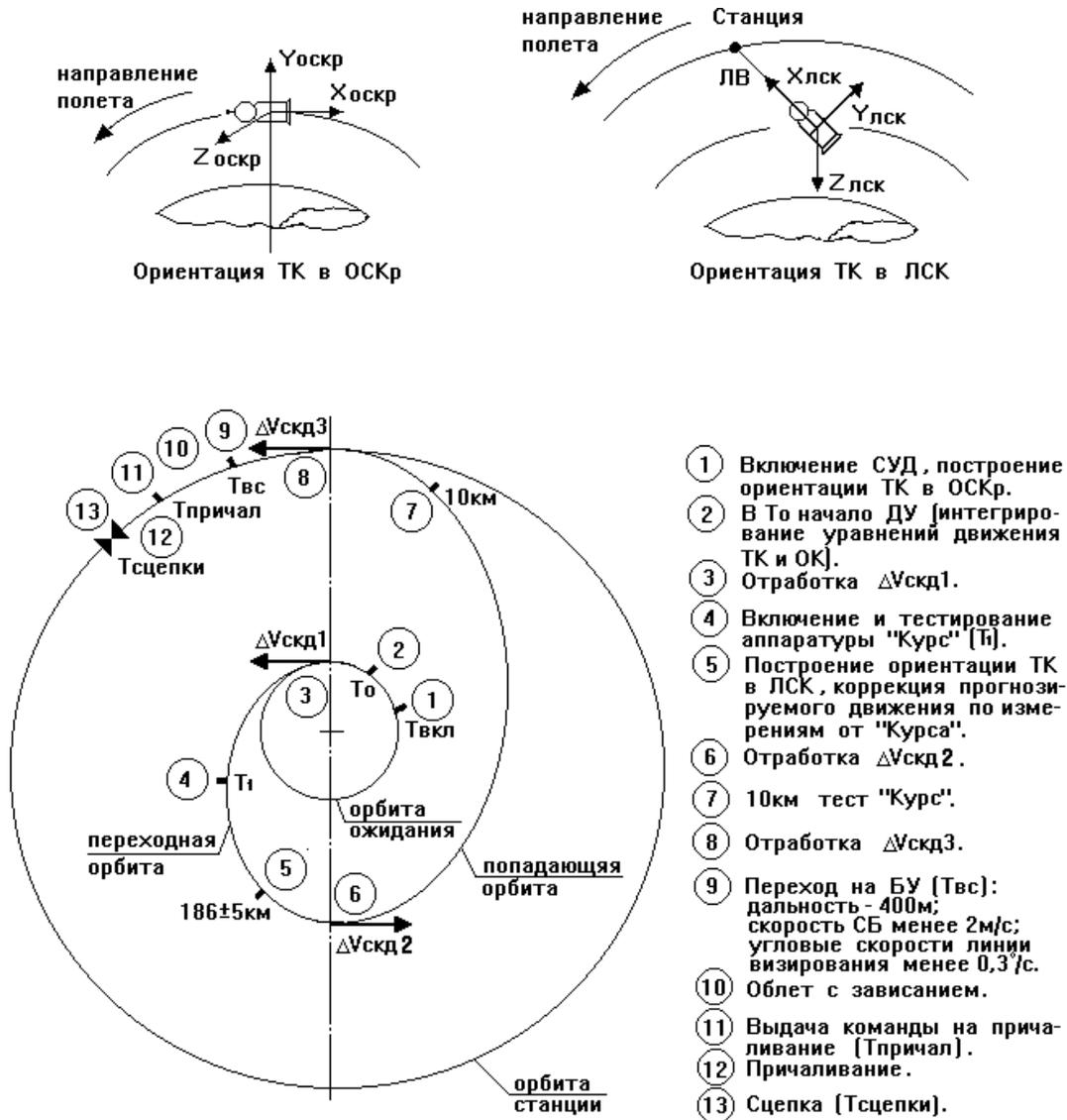
Fig. 2. (Spacecraft to Station Approach Cyclogram)
