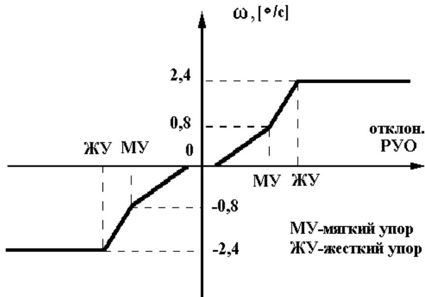
**Fig. 9. (PVO Attitude Control Characteristics in the AK Manual Mode)**
