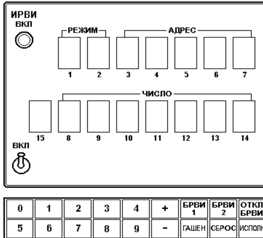
Fig.6. Manual Data Load Panel (ПРВИ)
