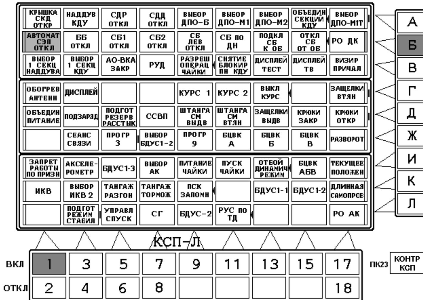
Fig.2. Command/Signal Panel - Left (КСП-Л)
