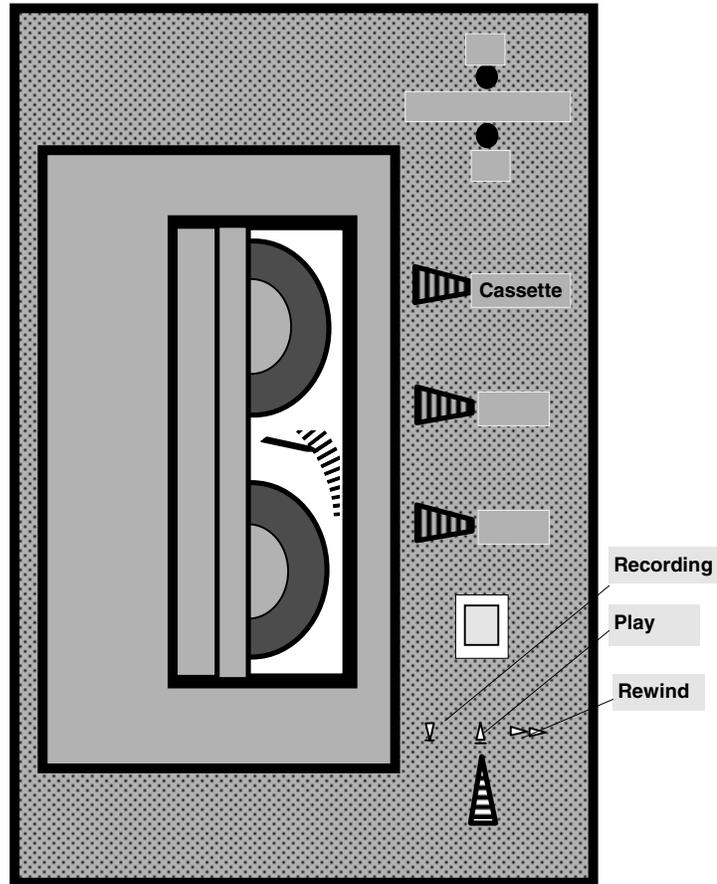
Fig. 4. "Gnom-S" Onboard Tape Recorder Exterior Appearance
