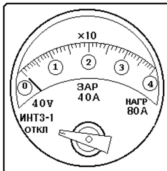
Fig.14. Voltage & Current Indicator (ИИТ)
