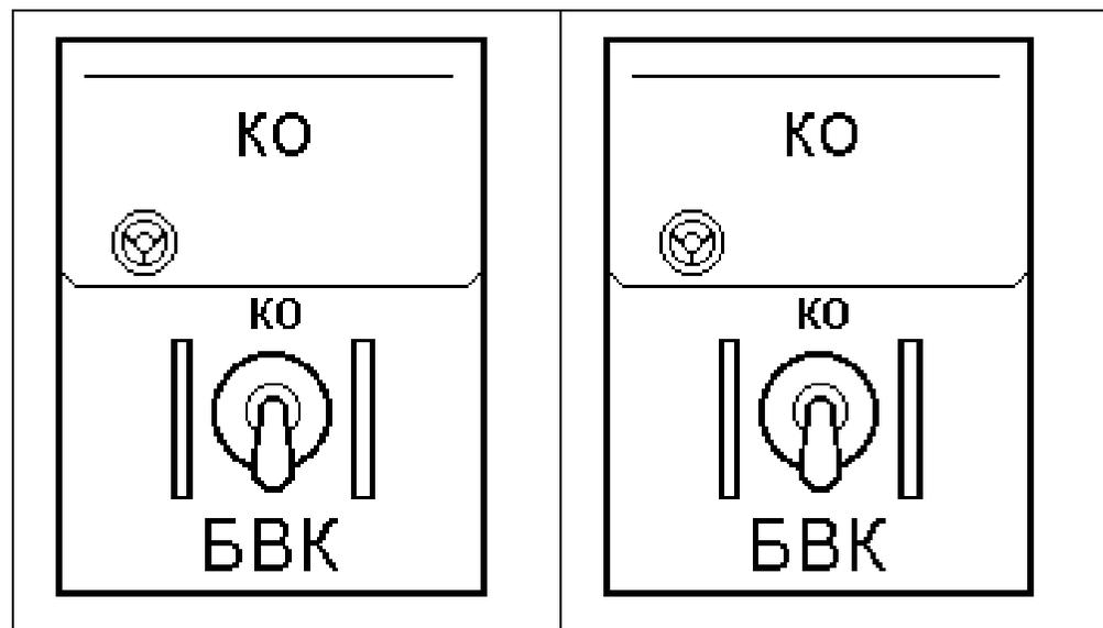
Fig.12. "Separation Contact" Command Issue Unit (БК)
