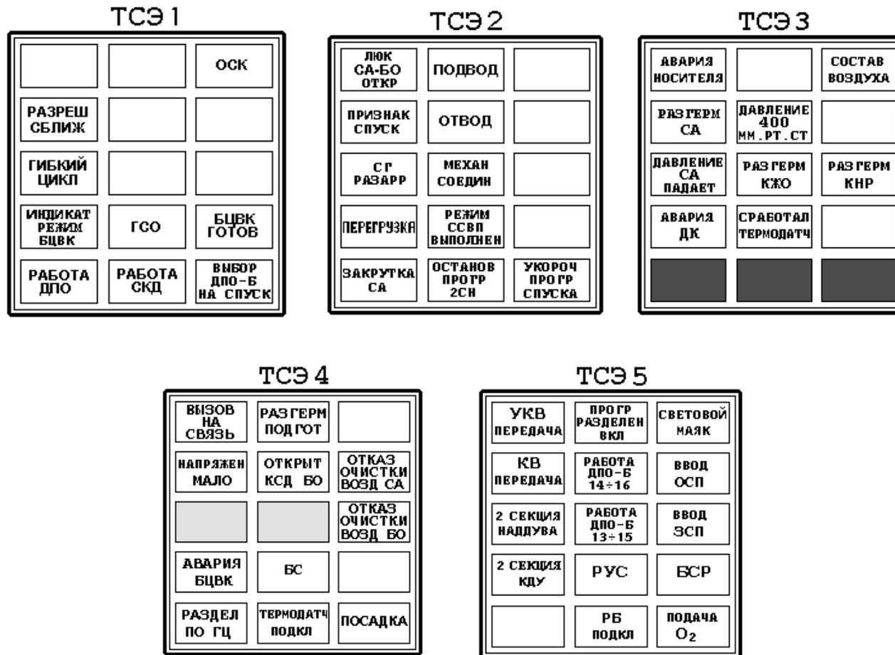
Fig.4. Electroluminescent Indicator Displays (ТСЭ)
