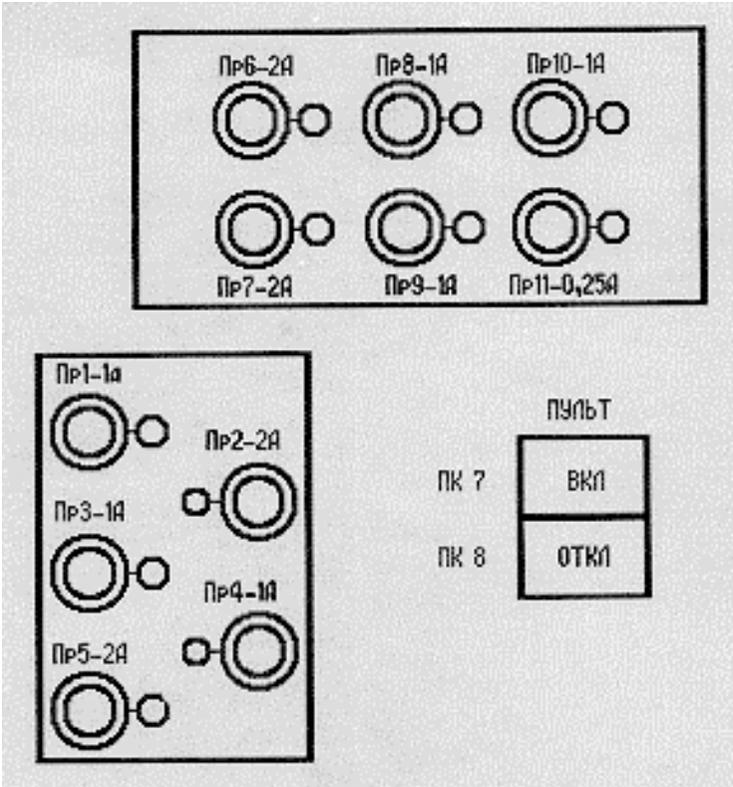
Fig.13. Circuit Breaker Sets and ПК CA Power Distribution
