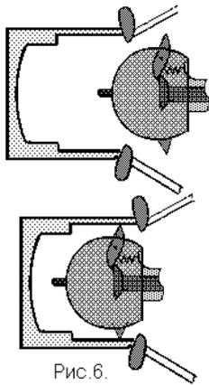
In the forward part of the CM Rod there are four Latches. The Latches can be in either of the two positions: extended or retracted, the extension and retraction being executed by the latch retraction mechanism driven by the Latch Actuator (ПЗ).
