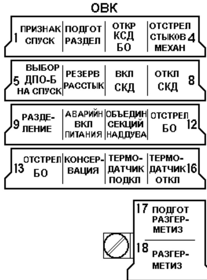
Fig.10. Critical Command Keys (ОВК)
