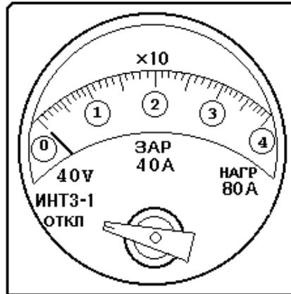
**Fig. 11. Voltage & Current Indicator**
