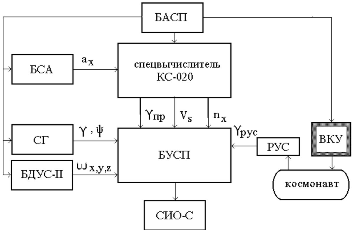
Fig. 1. (Descent Control Circuit Block Diagram)
