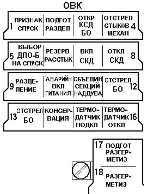
Fig. 7. OBK (Critical Command) Keys
