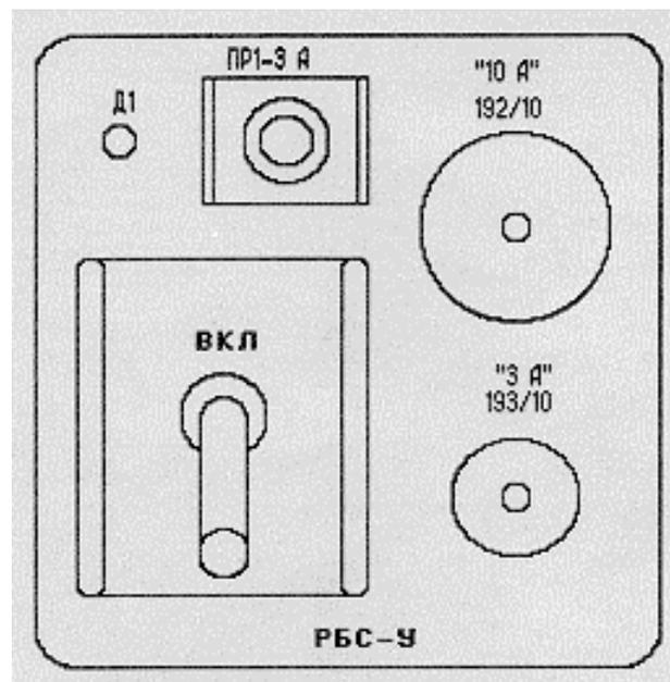
Fig.17. Universal Onboard Network Outlet (РБС-У)
