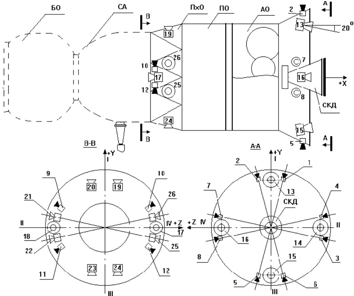
Fig. 1. (КДУ Thruster Location Layout)
