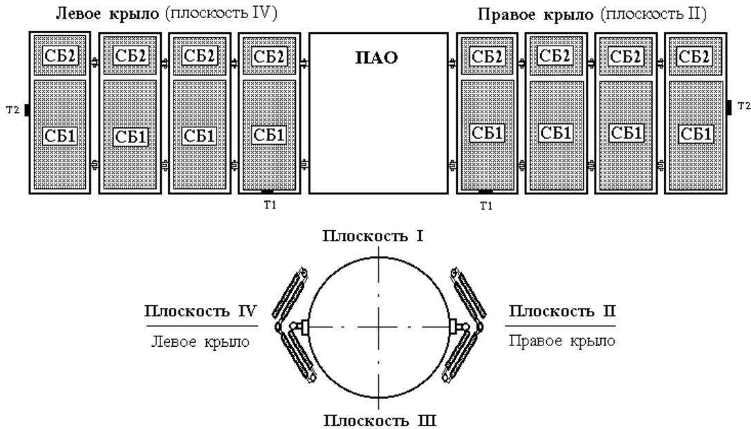
**Fig. 2. СБ Location and Structure**
