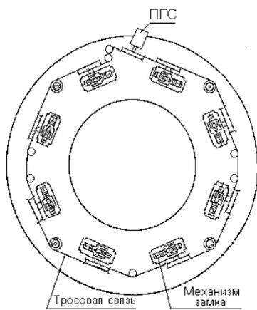
The МГС (Interface Pressurization Mechanism) is designed to ensure the second mechanical link, i. e. rigid and hermetically sealed connection of the spacecraft and station docked. The design of the АСА (Active Docking Assembly) МГС and the ПСА (Passive Docking Assembly) МГС is identical.
