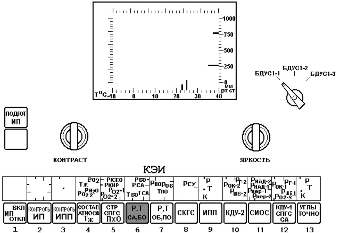
**Fig. 8. Combined Electronic Indicator**
