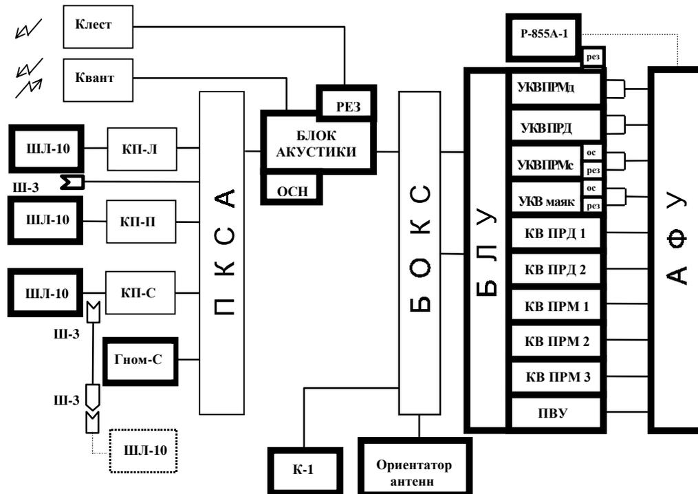
The VHF transmitter is designed for the crew communication with the ground and with Mir orbital station and for the CA Module direction finding signal transmission in the descent/landing phase.
